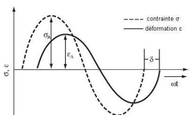
The complex Young modulus ( $E' + jE''$ ) is an essential parameter for the characterization and simulation of the acoustic behaviour of viscoelastic and porous materials.
